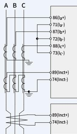
\*In case of using three winding CT as 3CT Y winding in the 3-phase 3-wire resistance grounding system
