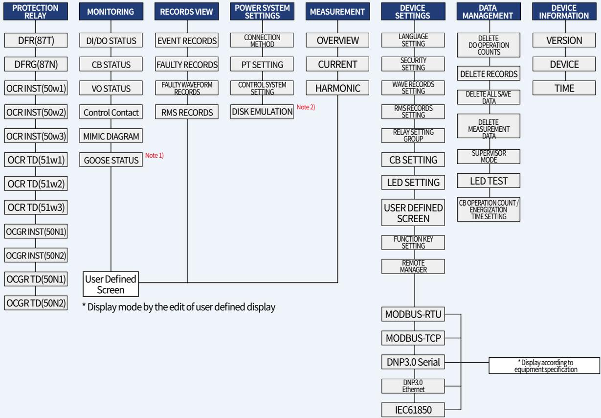
Note) 1. GOOSE reception status function: Refers to the function of displaying the reception status of the GOOSE message subscribed to in IEC 61850 communication.
