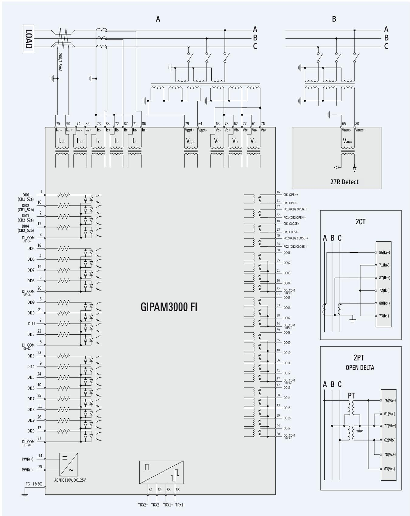
Note) GIPAM3000 recommends 3PT Y connection for optimal system protection.
