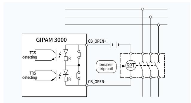
\* Terminal between the CB\_OPEN contactors may always have a resistance of around 200 kΩ, which may not operate normally when used for any purpose other than TRIP.
